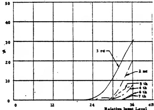
Fig. 6. Distortion components for two-stage pentode amplifier.
