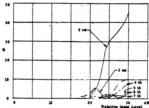
Fig. 8. Distortion components for multistage capacitor-coupled transistor amplifier.
